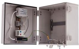
The AccelTex Solutions Heated PoE enclosure allows an access point to be installed in an outdoor or other temperature-limiting environment. The heater and AP are powered by a single PoE cable run from the network switch. The enclosure ships ready for an AP and external antenna installation.
